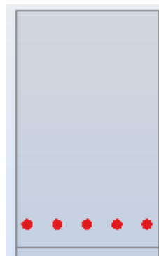
Fig. 5.2 Reinforcement (5φ20) assumed in [1]
